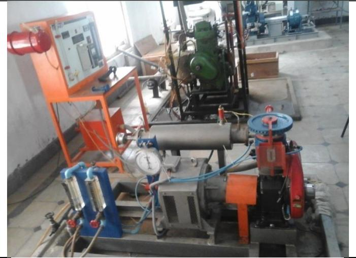
Computerized VCR Diesel engine test rig.
